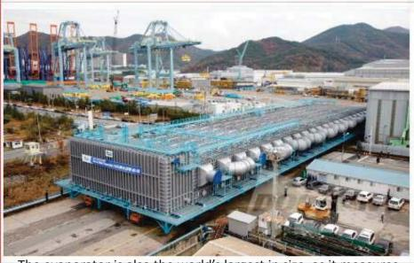
The evaporator is also the world's largest in size, as it measures 123 meters long, 33.7 meters wide, and weighs 4,150 tons
