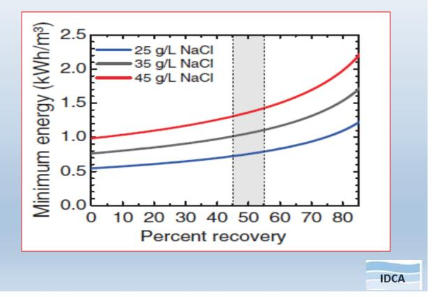
The theoretical minimum energy of desalination as a function of percent recovery can be obtained from the figure. As the salinity of seawater or desired water recovery increases, so does the minimum energy required for desalination.
