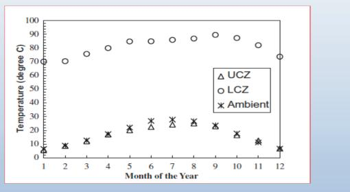
Annual temperature profile of the El Paso solar pond (UCZ –temperature of upper convective zone; LCZ – temperature of lower convective zone; ambient – temperature of ambient air).
